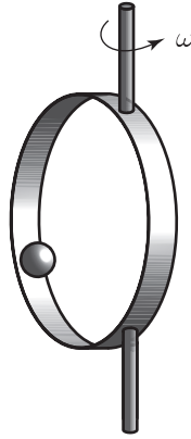
FIGURE 1.1.10. A ball in an off-center rotating hoop.
