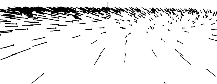
Fig. 3. Velocity field produced by combined translation and rotation, resulting from translating toward the vertical line while fixating the circle on the passing ground surface.
